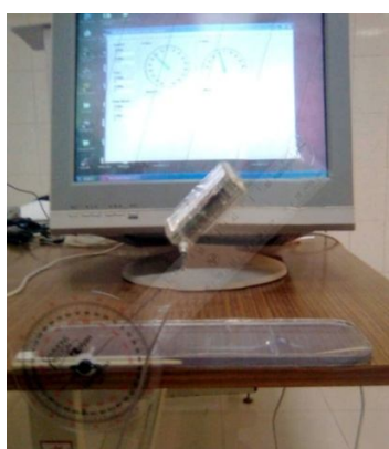
Figure 2: Virtual corset is placed on the movable arm of goniometer at the extension position
