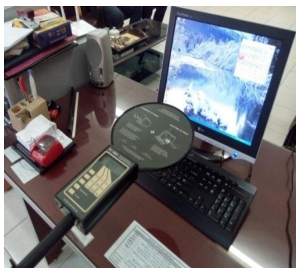
Figure 2. Gauss Meter Direction for Measuring the Magnetic Field
